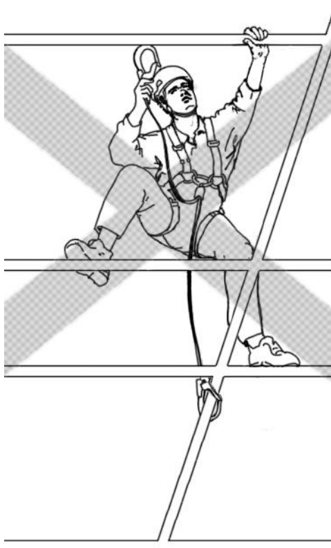
Figure Q.2 — Lifting an anchor sling from its normal hanging position increases the potential fall distance
